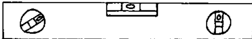
FIG. V-3. COMMERCIALY MANUFACTURED LEVEL
